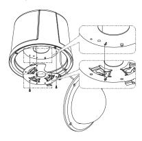
Connect the safety cable from the housing to the internal fixture ring of the STH-270PWV wall mount.
